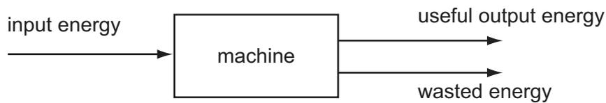
The machine is 50% efficient.
